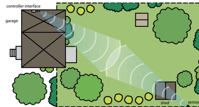
Two-way messaging allows the system to overcome most line-of-site obstructions, such as trees, sheds and even walls.
