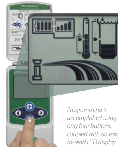
Programming is accomplished using only four buttons, coupled with an easy-to-read LCD display.
